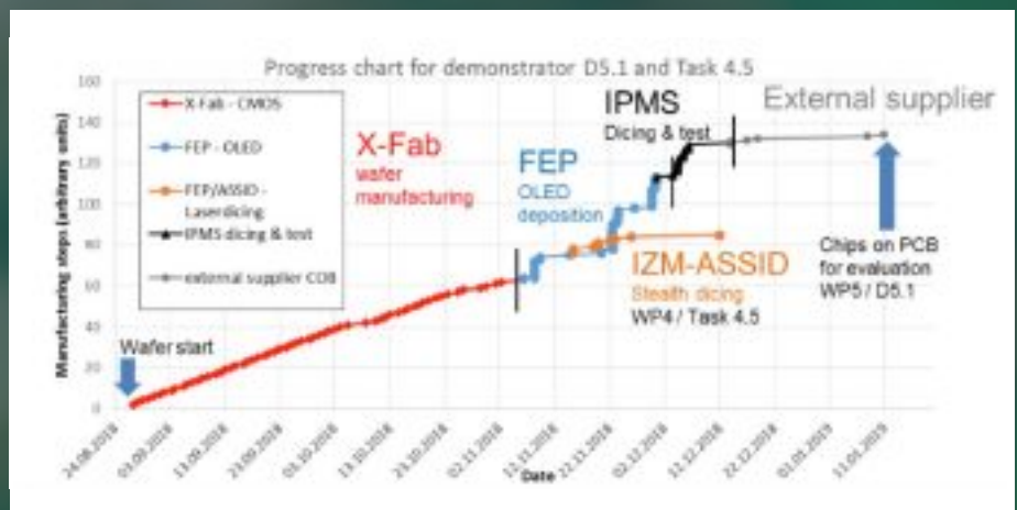
Figure 3. Logistics and added value along the ADMONT pilot line with external supplier
